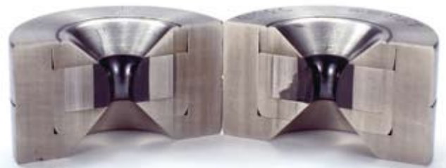
Cross section of wire twisting dies
