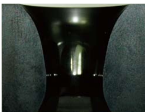
Cross section (along the length of die hole) of a sintered diamond die
